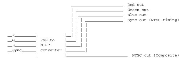
The converters discussed below use this approach to drive both a RGB device and a NTSC device with the same video image simultaneously.
