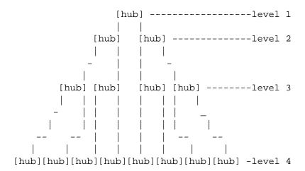
Whether the cascaded hub configuration is a better design than the backbone depends on several factors.
