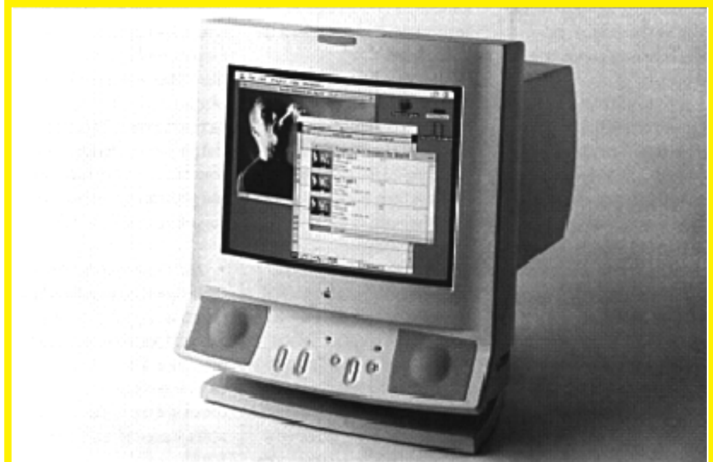
The Apple AudioVision 14 Display, the first computer display with integrated audio and video capabilities.
